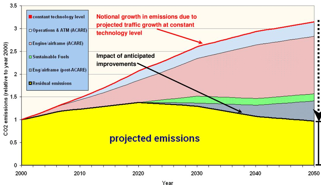
Figure 2: SA CO<sub>2</sub> Roadmap - projected future emissions of CO<sub>2</sub> from UK aviation
