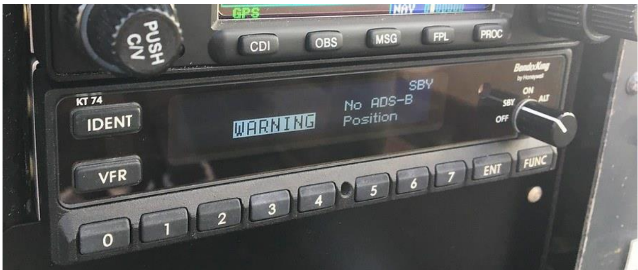
Figure 9: Photograph of KT74 transponder in AC5 indicating “No ADS-B Position”
